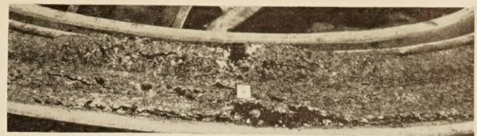
FIGURE 2.—APPEARANCE OF SECTION 4 AT 40,572 WHEEL-TRIPS, OR 572 WHEEL-TRIPS AFTER START OF TESTING WITH CONCENTRATED TRAFFIC.
